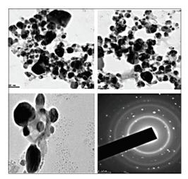
Figure 5: Transmission electron microscopy analysis of silver nanoparticles synthesized *Abutilon indicum*
