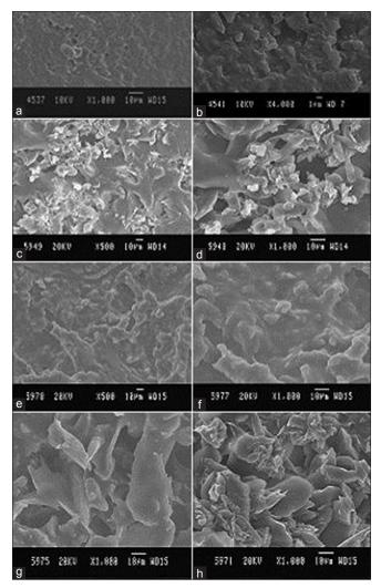
Figure 6: Scanning electron micrographs: Blank implants immediately after manufacturing [a(B1) and b(B2)], Blank implants after 30 days release [c(B1) and d(B2)], PTX loaded implants immediately after manufacturing [e(F1) and f(F2)] and PTX loaded implants after 30 days release [g(F1) and h(F2)]
