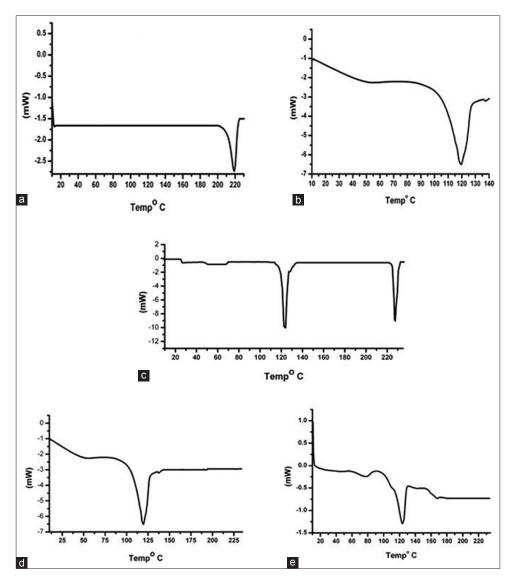
Figure 3: DSC thermograms of pure PTX (a), poly(SA-RA) (b), physical mixture of drug and polymer (c), F1 (d) and F2 (e). The experiment was carried with crimped aluminum pans and a heating rate of 10°C/min; the samples were scanned at 10°C/min from 10-225°C
