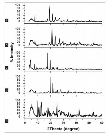
Figure 4: XRD patterns of pure TC (a), poly(SA-RA) 70:30 w/w (b), physical mixture (c), F1 (d) and F2 (e)
