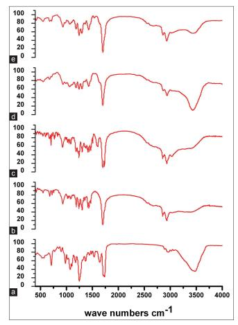
**Figure 2:** Transmission FT-IR spectra of pure PTX (a), poly(SA-RA) (b), physical mixture of PTX and poly(SA-RA) (c), F1 (d) and F2 (e)
