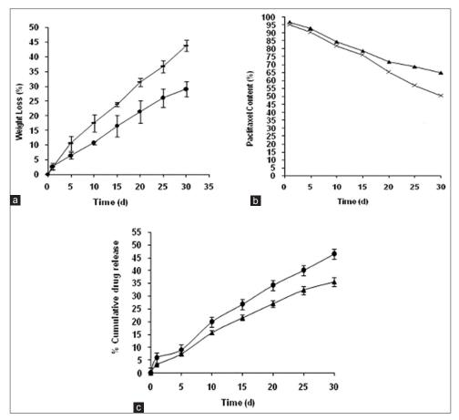
Figure 5: (a) In vitro hydrolytic degradation of percentage weight loss of drug loaded implants F1 (•) and F2 (•), (b) Paclitaxel content (accumulated) during hydrolytic degradation F1 (▲) and F2 (x), (c) Percentage cumulative drug release F1 (•) and F2 (▲), respectively
