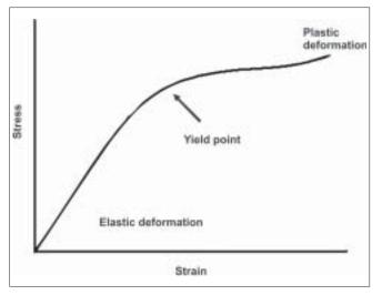
Figure 1: Stress strain curve for a solid
