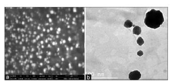
**Figure 3:** Photomicrographs of doxorubicin-solid lipid nanoparticles obtained by (a) scanning electron microscopy (b) transmission electron microscopy
