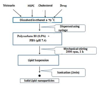
Figure 1: Schematic representation of the method of preparation of solid lipid nanoparticles
