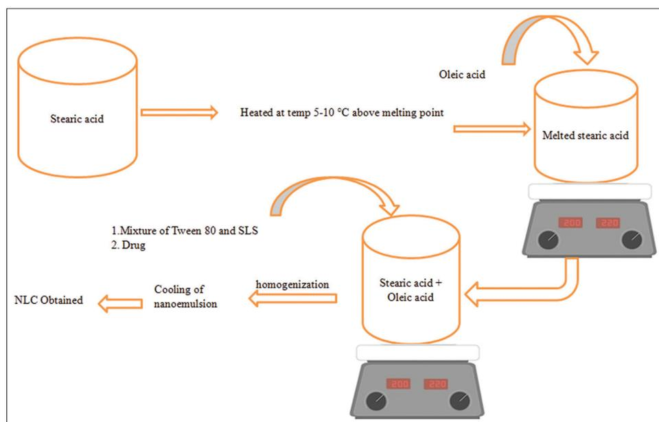
Figure 1: Schematic presentation of NLC formulation
