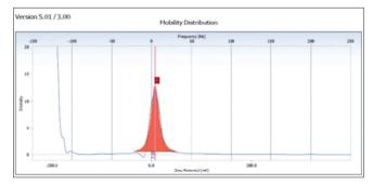
**Figure 6:** Zeta potential of silver nanoparticles: Glucose and poly vinyl pyrrolidone K30
