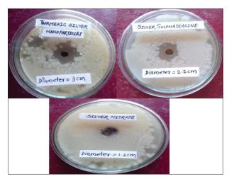
**Figure 8:** Zone of Inhibition of silver nanoparticles: Turmeric and silver sulphadiazine plain drug and silver nitrate
