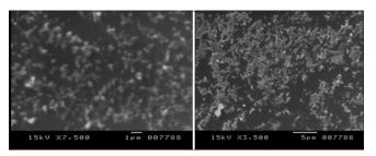
**Figure 4:** Scanning electron microscopy images of silver nanoparticles: Glucose and poly vinyl pyrrolidone K30
