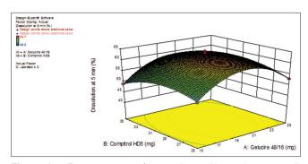
**Figure 2:** Response surface plots (three-dimensional) showing the effect of the amounts of Gelucire 48/16 ( $X_1$ ) and Compitrol HD5 ( $X_2$ ) added on the response  $Y_2$  (dissolution after 5 min)
