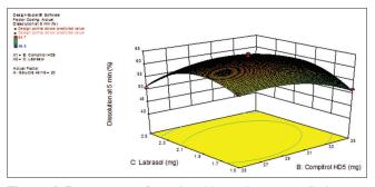
**Figure 4:** Response surface plots (three-dimensional) showing the effect of the amounts of Compitrol HD5 ( $X_2$ ) and Labrasol ( $X_3$ ) added on the response  $Y_2$  (dissolution after 5 min)
