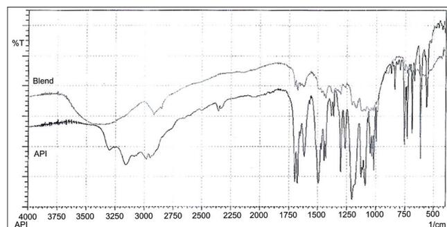
Figure 5: Comparative infrared spectra between amlodipine besylate and blend
