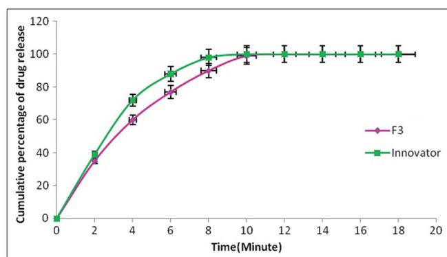
Figure 2: Comparative *in vitro* dissolution study between best batch (F3) and innovator
