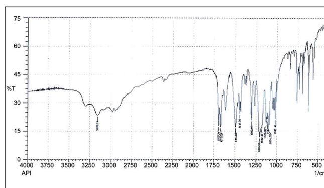
Figure 3: Infrared spectra of amlodipine besylate
