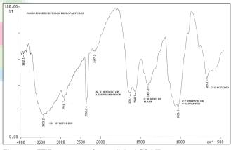
Figure 4: FTIR spectrum of cross-linked CS MPs
