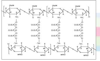
Figure 7b: Schematic representation of ionic cross linking
