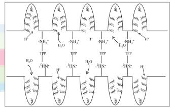
Figure 9: Schematic depiction of lower cross-linked CS bead-acid resistive property
