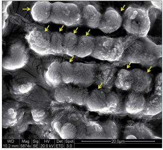
Figure 7a: SEM image showing cleaves at the weak sites of CS beaded chains (represented by arrow marks)
