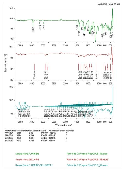
Figure 1: A typical infrared spectra of Gelucire 50/13 and physical mixtures of flutamide and Gelucire 50/13 in ratio 1:2
