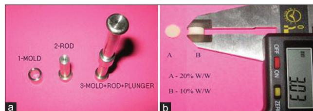
**Figure 1:** Designed and fabricated molds for preparation of implants (a) and formulation (b)
