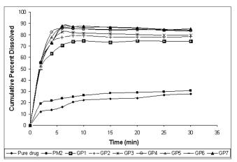
Figure 3: Cumulative percent release of glimepiride from solid dispersions and physical mixtures of glimepiride-poloxamer 188 systems
