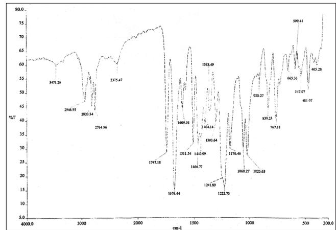
**Figure 2:** IR spectrum of diltiazem base
