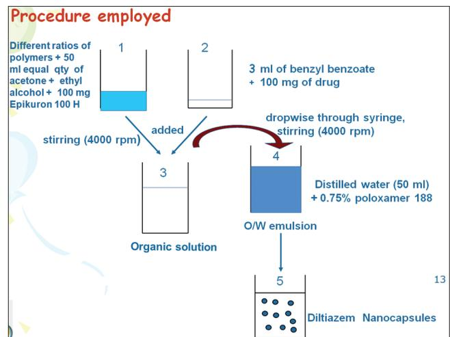
**Figure 3:** Preparation of nanocapsules
