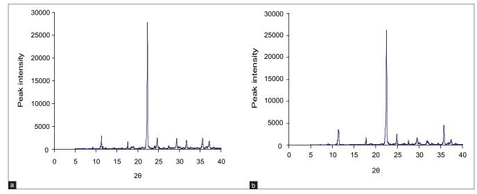
Figure 1: X-ray diffractogram of PM and HSD; (a) 1 : 10 PM (b) 1 : 10 HSD
