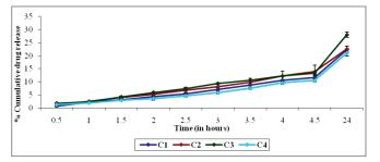
Figure 7: Effect of concentration of CaCl2 of microspheres on dissolution rate of DF-loaded alginate microspheres
