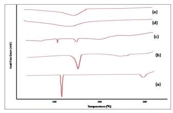
Figure 3: DSC thermogram of (a) diloxanide furoate (DF; Drug) (b) alginate (Polymer) (c) mixture of DF and alginate (d) alginate microspheres without drug (e) alginate microspheres loaded with drug
