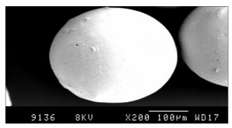
Figure 2: SEM photomicrograph of diloxanide furoate-loaded alginate microspheres
