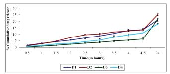
Figure 8: Effect of stirring rate of microspheres on dissolution rate of DF-loaded alginate microspheres
