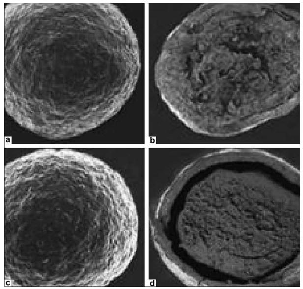
Figure 1: Scanning electron micrographs of pectin–HPMC (1:3) coated pellets: (a) coated pellet (surface); (b) cross-section; (c) After 12-hour incubation in control phosphate buffer conditions (surface); (d) cross section
