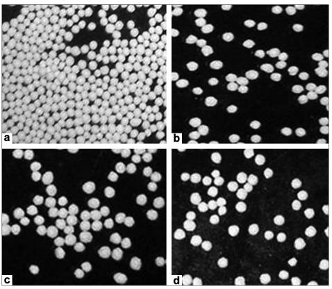
Figure 1: Drug loaded beads (dried, 18/24 size) prepared by extrusion-spheronization technique (a: Core beads; b: Eudragit RL 30 D, c: Eudragit RS 30 D, d: Eudragit NE 30 D coated pellets)
