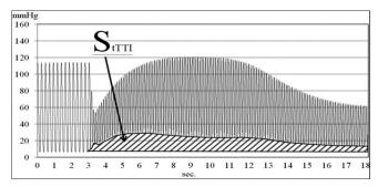
**Figure 2:** Stress test with submaximal electrical stimulation in Langendorff heart of rats with DOX-induced cardiomyopathy. Dynamic of pressure in the left ventricle (mmHg) with high-rate stimulation of the heart (480 bmp) for 15 s. The intact group
