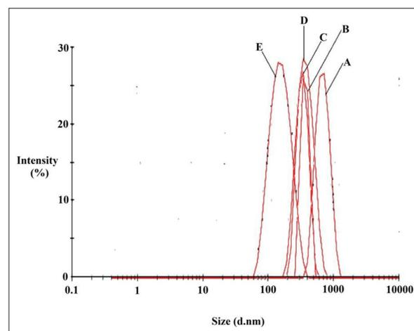
**Figure 2:** Nanoparticles size distribution by intensity (Batch – A, B, C, D, and E)
