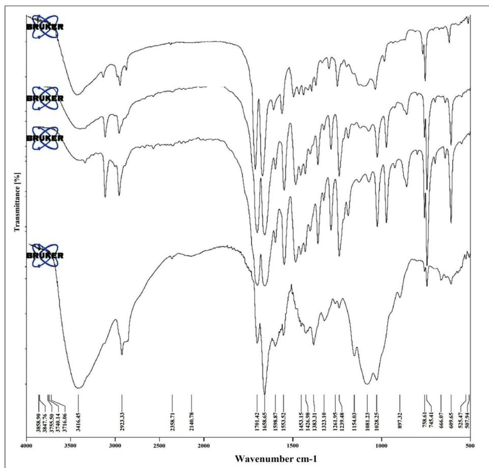
**Figure 1:** FT-IR spectra (A) Low-molecular-weight chitosan (LMC); (B) caffeine; (C) LMC + Caffeine; and (D) caffeine-loaded LMC carrying nanoparticles
