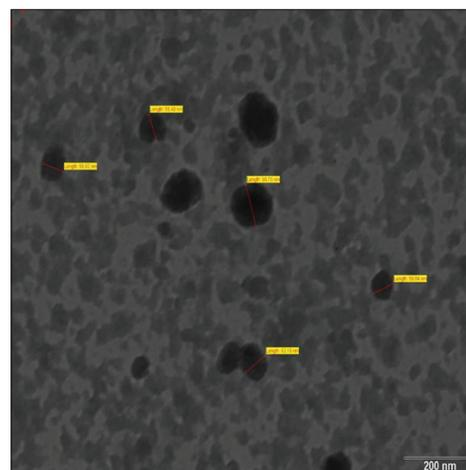
**Figure 3:** Transmission electron microscopy image of caffeine-loaded nanoparticles
