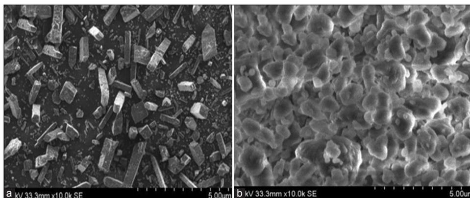
Figure 3: (a) Scanning electron microscopy (SEM) of clomiphene citrate, (b) SEM of liquisolid formulation
