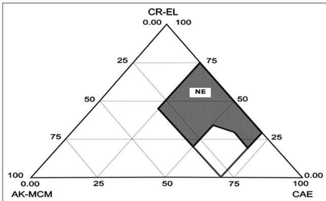
Figure 1: Ternary phase diagram of CR-EL, AK-MCM and capryol 90
