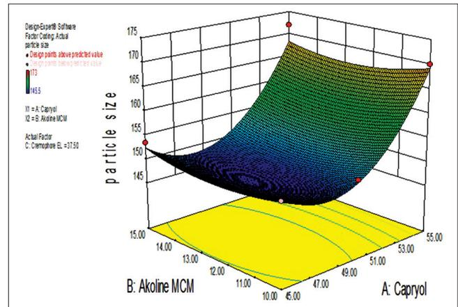
Figure 4: Response surface plot for particle size (Cremophore EL = 37.50%)
