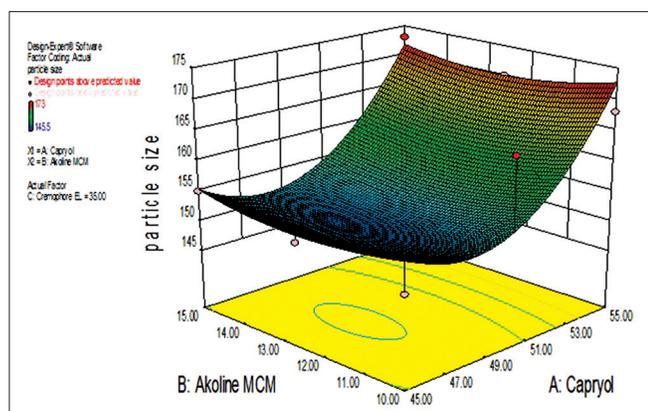
**Figure 5:** Response surface plot for particle size (Cremophore EL = 35%)
