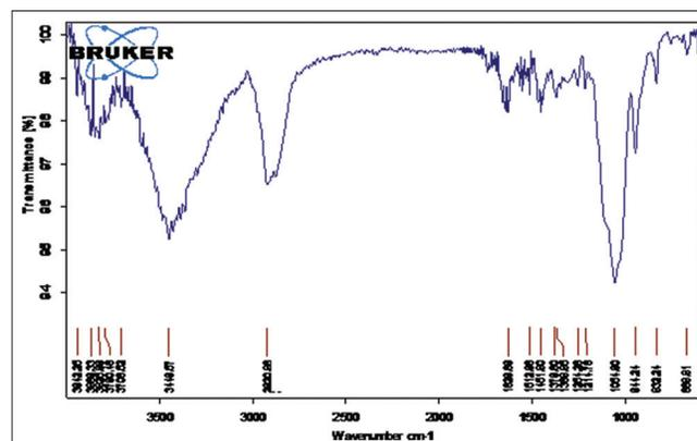
Figure 3: FT-IR spectra of optimized liquisolid formulation (F8)
