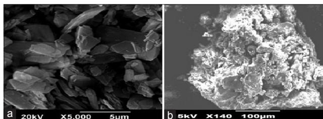
**Figure 4:** Scanning electronmicroscopy picture of (a) pure drug (carvedilol), (b) inclusion complex (carvedilol-HP $\beta$ -CD)
