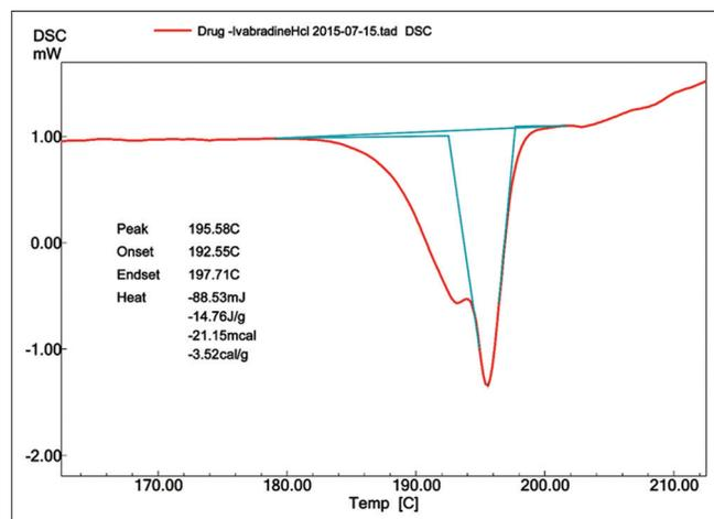
**Figure 4:** Differential scanning calorimetry thermogram of ivabradine Hydrochloride
