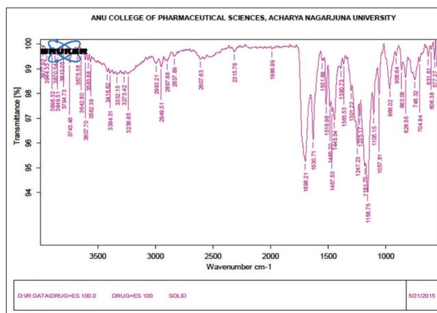
**Figure 1:** Fourier transform infrared spectroscopy spectrum of physical mixture of ivabradine Hydrochloride and Eudragit S100
