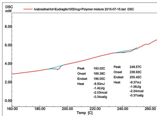
**Figure 3:** Differential scanning calorimetry thermogram of ivabradine Hydrochloride and Eudragit S100
