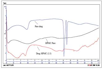
**Figure 11:** Overlaying of differential scanning calorimetry thermograms of drug, polymer and solid dispersion of hydroxy propyl methyl cellulose E15
