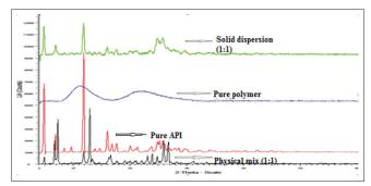
**Figure 8:** Overlaying of powder X-ray diffraction patterns of various compounds of poly vinyl pyrrolidone K30
