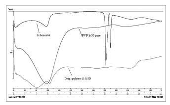
**Figure 10:** Overlaying of differential scanning calorimetry thermograms of drug, polymer, and solid dispersion of poly vinyl pyrrolidone K30
