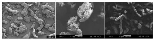
Figure 13: Scanning electron microscopy of hydroxy propyl methyl cellulose E15, solid dispersion of 1:3 ratio and physical mixture of 1:3 ratio
