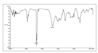
**Figure 6:** Fourier transform infrared spectra of solid dispersions of poly vinyl pyrrolidone k30 (1:1 ratio)
