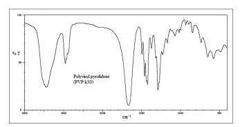
**Figure 4:** Fourier transform infrared spectra of poly vinyl pyrrolidone K30
