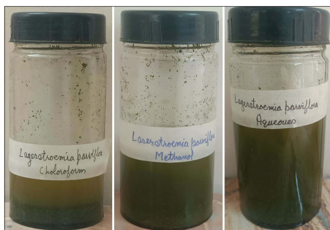
Figure 2: Extraction of plant leaves by the maceration process
