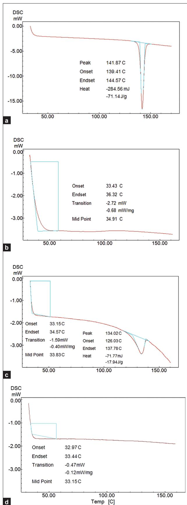
**Figure 3:** DSC thermogram of (a) SV, (b) PLGA, (c) SV/PLGA physical mixture, and (d) SV-loaded PLGA nanoparticles
