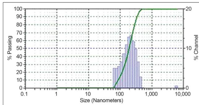
**Figure 1:** Laser light scattering the particle size histogram of optimized SV-loaded PLGA nanoparticles prepared by using dichloromethane as an organic solvent, drug polymer ratio 1:2, and PVA as a stabilizer
