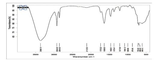
Figure 5: Fourier transform infrared spectrum of Benzalkonium chloride
