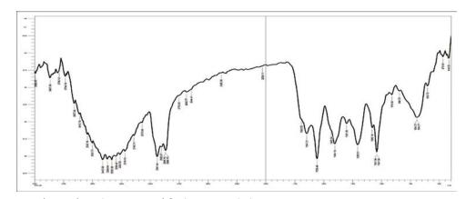
Figure 8: Fourier transform infrared spectrum of Sodium tourocholate
