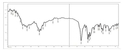
Figure 7: Fourier transform infrared spectrum of Disodium EDTA
