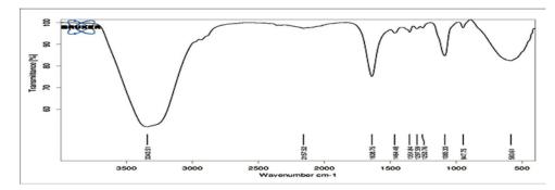
Figure 26: Fourier transform infrared spectrum of optimized formulation (F2)
