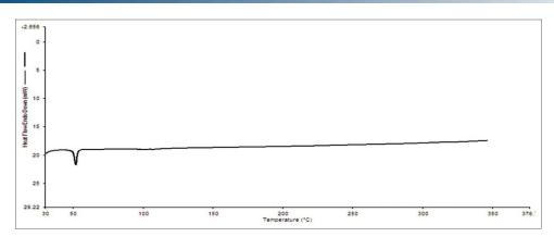
**Figure 11:** Differential scanning calorimetry thermogram of F11 optimized formulation (Hydroxyl propyl methyl cellulose K4M: Sodium tourocholate [0.5% w/v: 0.5% w/v])
