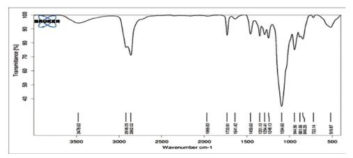
Figure 6: Fourier transform infrared spectrum of Tween 20
