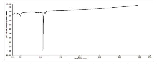
**Figure 9:** Differential scanning calorimetry thermogram of F2 optimized formulation (Hydroxyl propyl methyl cellulose K4M: Tween 20 [0.5% w/v: 0.5%v/v])
