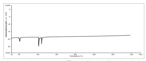
**Figure 10:** Differential scanning calorimetry thermogram of F5 optimized formulation (Hydroxyl propyl methyl cellulose K4M: Disodium EDTA [0.5% w/v: 0.5% w/v])
