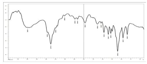
Figure 3: Fourier transform infrared spectrum of Poloxamer 407
